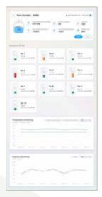
**Simplified Visuals:** Quickly view the temperatures, capacity, battery level and alarms. Devices can be remotely controlled and quickly located; features include remote single/batch unlocking, and "Find My Tank".
