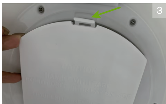
Figure 2-12 Battery replacement: Ejection (left 3 figures) and Insertion (right 3 figures)
